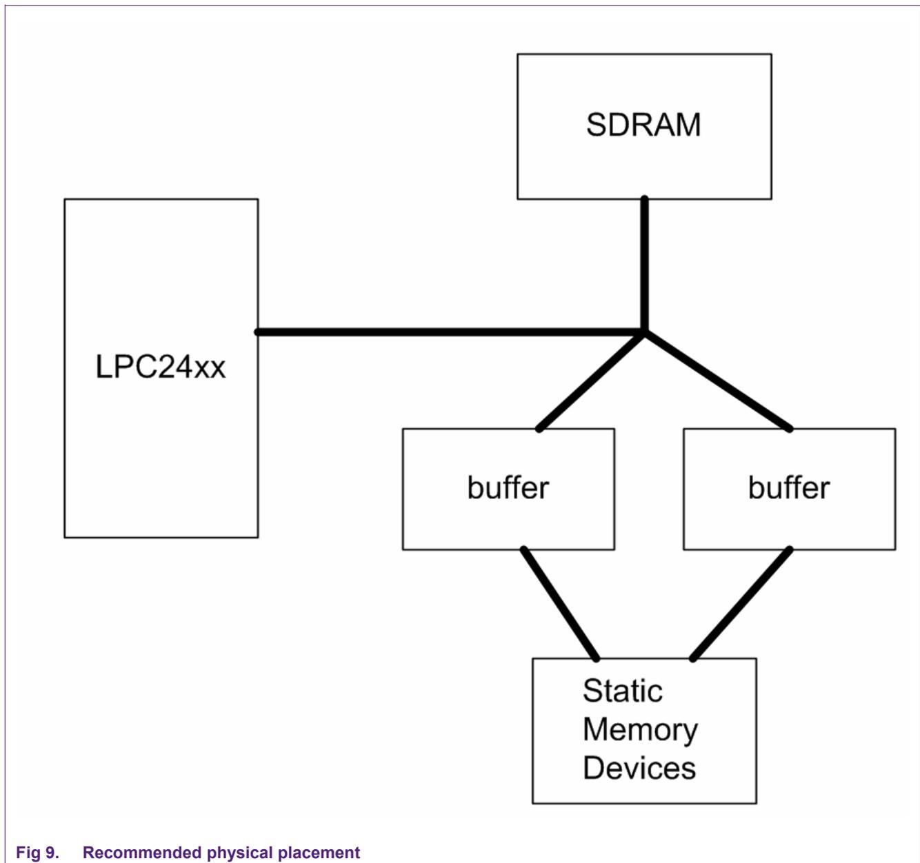
Fig 9. Recommended physical placement
