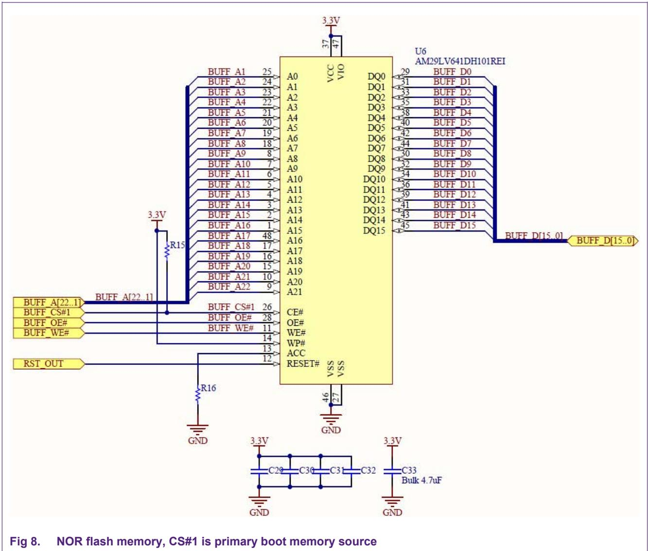
Fig 8. NOR flash memory, CS#1 is primary boot memory source
