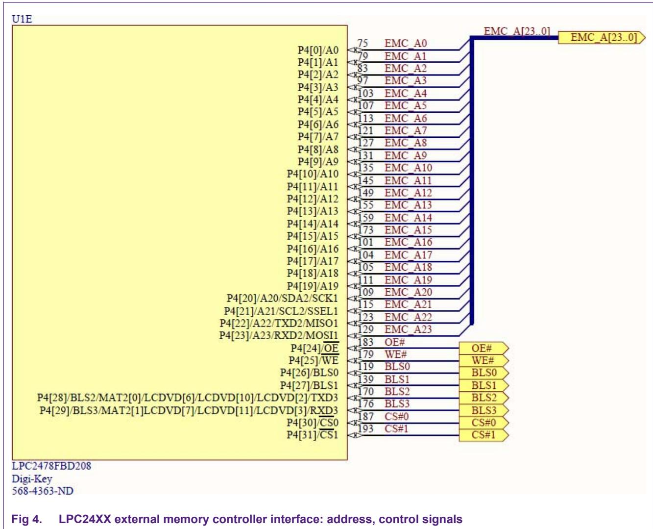
Fig 4. LPC24XX external memory controller interface: address, control signals
