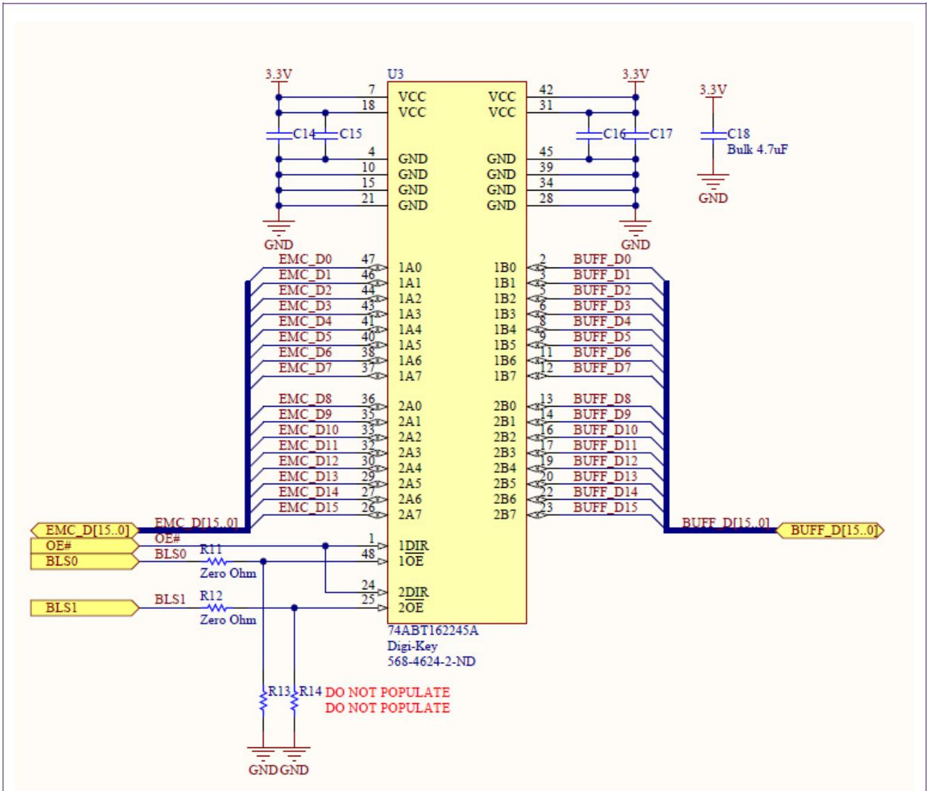
Fig 6. Data[15:0] buffering, BLS[1:0] control output enable
