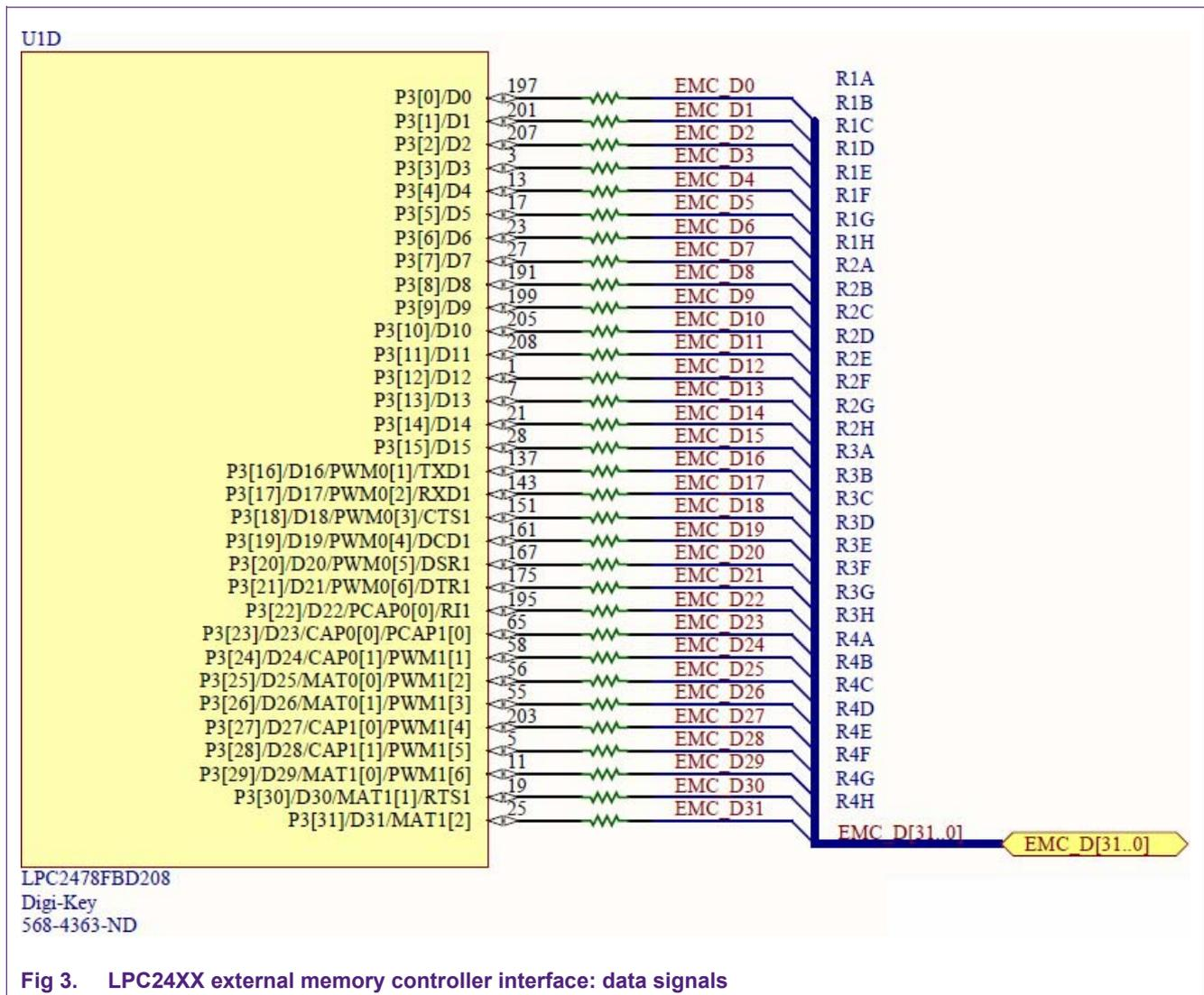
Fig 3. LPC24XX external memory controller interface: data signals
