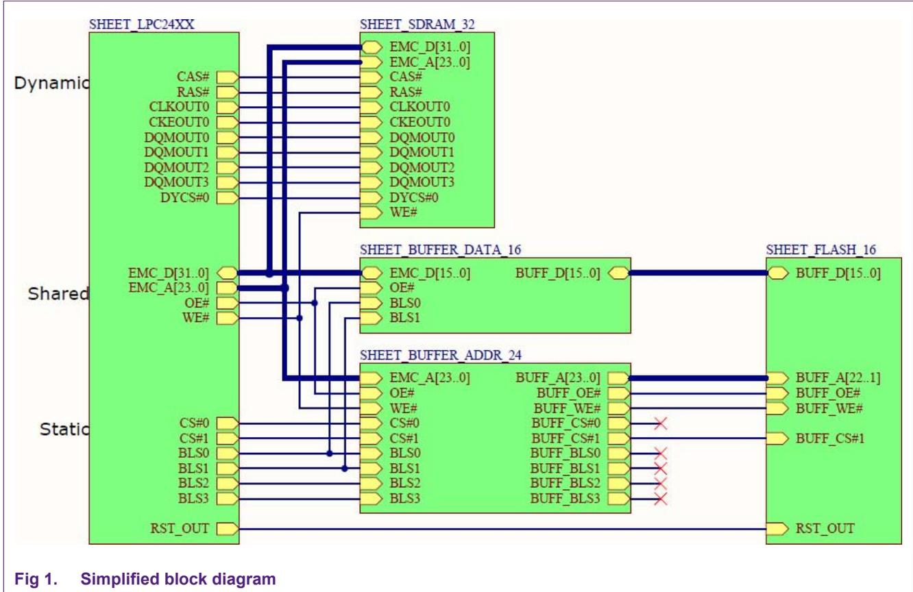
Fig 1. Simplified block diagram
