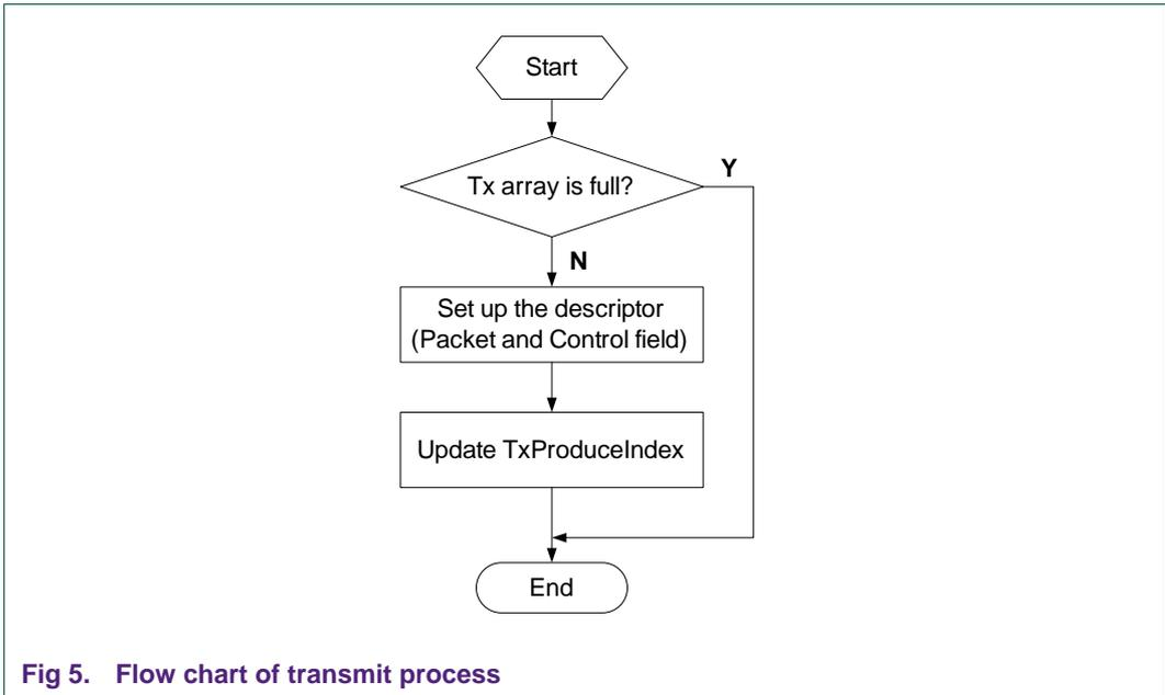
**Note:** If the transmit datapath is enabled the Ethernet block will start transmitting the frame as soon as it detects the TxProduceIndex is not equal to TxConsumeIndex - both were zero after reset.
